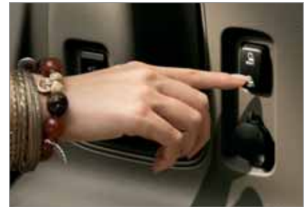
An available EasyFold™ rear seatback release lets you create a flat cargo loadfloor in seconds by simply pushing and holding a button in the rear cargo area.
