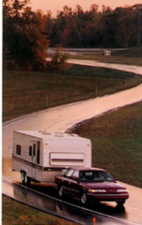
Crown Victoria's big towing capability is partially due to its rugged body-on-frame design. With the optional trailer towing package, capability is 5,000 lbs. — 2½ tons.
