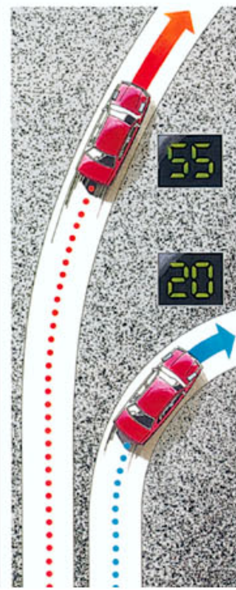
Speed-sensitive steering adjusts the degree of power assist according to the circumstances: maximum assist for low-speed maneuvers, progressively less for a better road feel at higher speeds.
