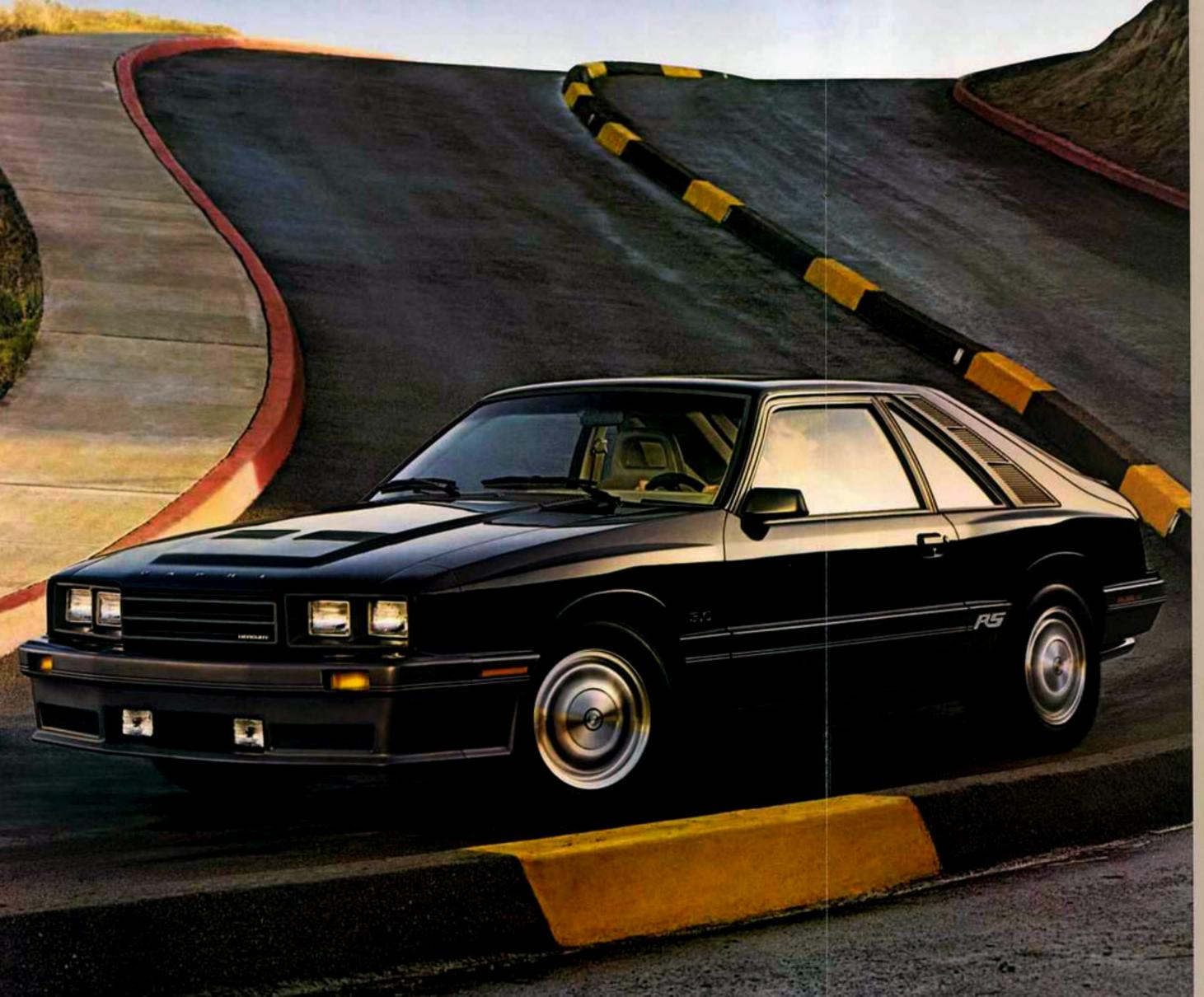
opri RS gets its might from a standard 5.0-liter High-Output four-barrel V-8 engine with five-speed overdrive manual transmission. This small block V-8 cranks out an impressive 210 horse-power at 4800 rpm.\* It yellow-lines at 5200 rpm and red-lines at 5800 rpm. It's the stuff of which dreams are made.
