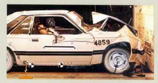
The doors on Capri feature strong ouble-panel welded construction. Inside ach door is a high-strength steel beam hich enables each door to withstand test load twice as great as Capri's urb weight.
